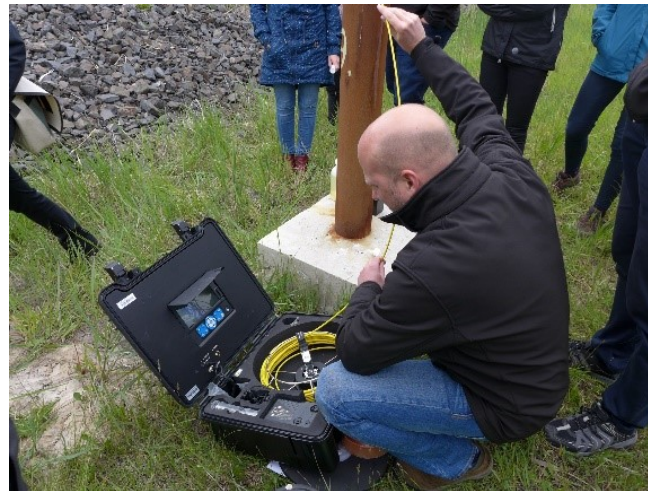
Demonstration of a monitoring well camera drive at Lake Most during the GeoMAP-Workshop at 15 May 2019
