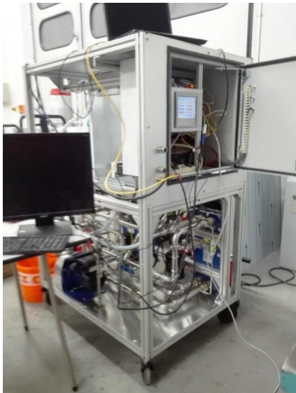
Mobile heat pump pilot rig, developed at the Department for Technical Thermodynamics.
